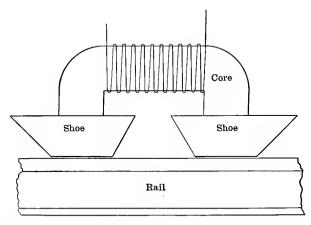
FIG. 51. Diagram of Westinghouse magnetic brake, showing several parts of the magnetic circuit.
